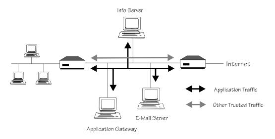
Figure 3.4: Screened Subnet Firewall with Additional Systems.
