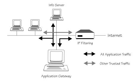
Figure 3.3: Screened Host Firewall.
