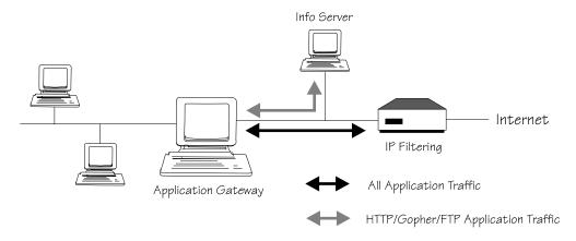
Figure 3.2: Dual-homed Gateway Firewall with Router.
