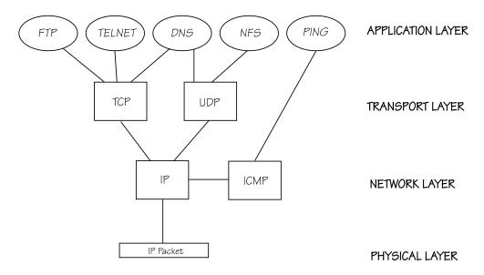
Figure 1.1: Conceptual View of Services and Layers in TCP/IP.
