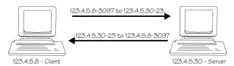
Figure 1.2: TELNET Port, IP Interaction.
