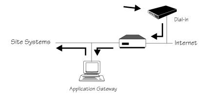
Figure 3.5: Modem Pool Placement with Screened Host Firewall.
