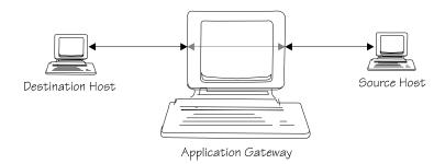
Figure 2.4: Virtual Connection Implemented by an Application Gateway and Proxy Services.
